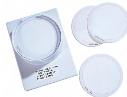
PM 2.5 Air Monitoring Membrane Filters
